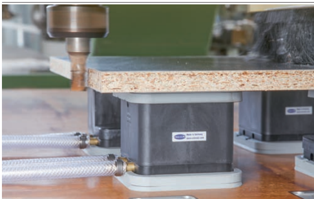
Vacuum blocks VCBL-G-K2 for clamping particle boards
