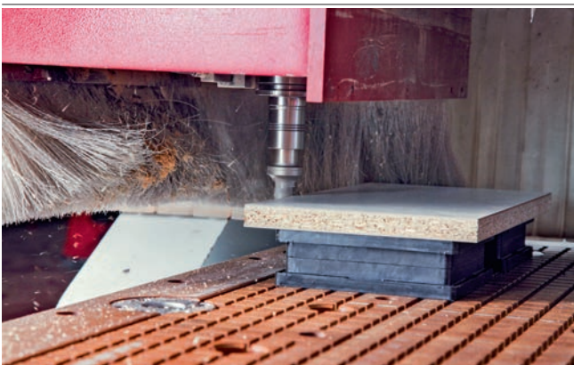
Vacuum blocks VCBL-R for clamping particle boards
