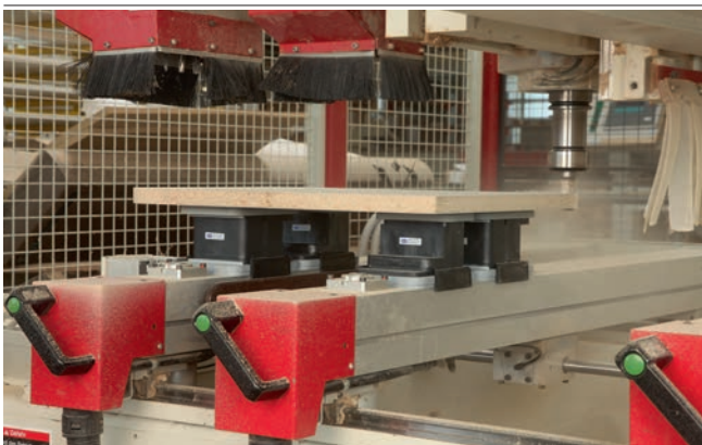
Vacuum blocks VCBL-K2 for clamping a workpiece
