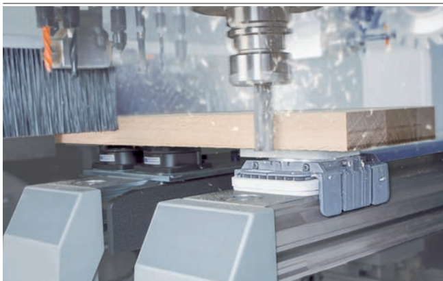
Vacuum blocks VCBL-K1 for clamping solid wood
