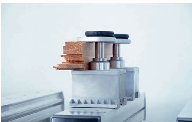
Mechanical clamps VCMC-K1-QUICK for clamping of frame parts
