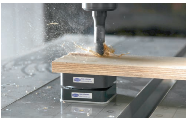
Innospann Cup and Mono-Base while clamping a wooden workpiece
