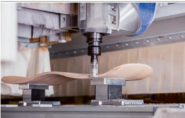
Aluminum vacuum blocks VCBL-A-K2 for clamping solid wood
