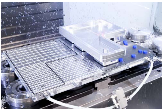
Modular design of the Matrix-Plate clamping system allows multiple setups on one fixture without retooling
