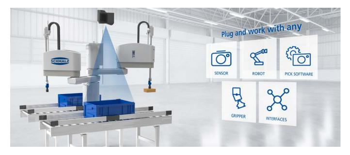
With ivOS, Schmalz has developed an operating system for bin picking. Integrators and machine builders receive an overarching, intelligent system that allows them to easily connect and control grippers, cameras, picking software and robots from different manufacturers. Modern interfaces enable comprehensive data exchange in real time, for example with warehouse management systems.
