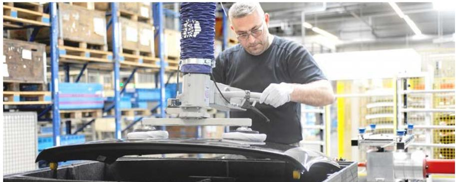
operating elements and grippers and are each designed for specific applications. This makes the vacuum tube lifter not only an ideal helper for machine loading, shipping and order picking
