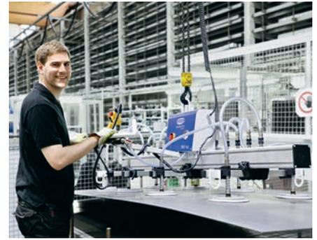
VacuMaster. With the ergonomic operator handle, the user maintains the required safety distance from the picked-up object and transports it to its destination safely, gently and without exerting force. Unlike the Jumbo, the VacuMaster only holds the workpieces. The lifting movement is performed by a chain hoist.
