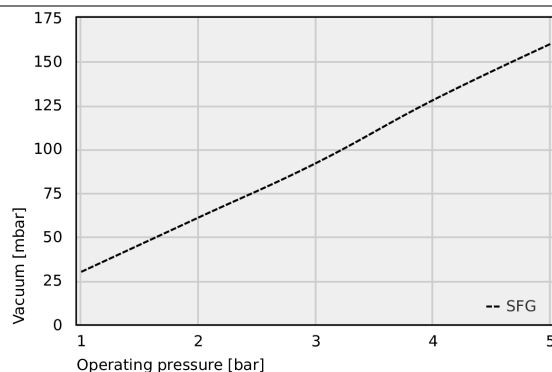
Achievable vacuum at various operating pressures
