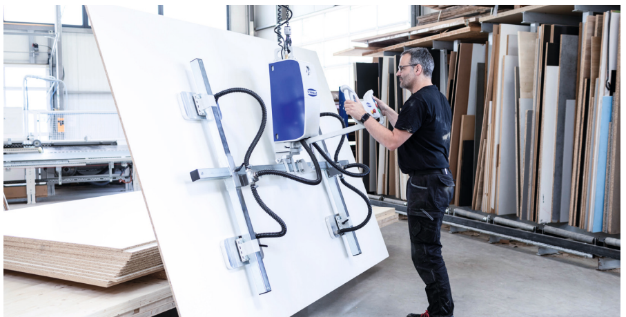
Vacuum lifter for heavy wooden boards
