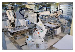
Vacuum Suction Spider SSP in the framing station
