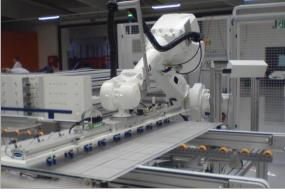
Bellows Suction Pads FG 19 used for layup of strings
