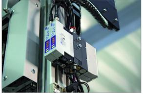
Compact Ejector for the vacuum supply for flipping stations of strings
