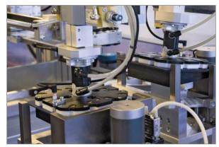
**Wafer Gripper SWG** used for the destacking of cells for the loading a stringer:
