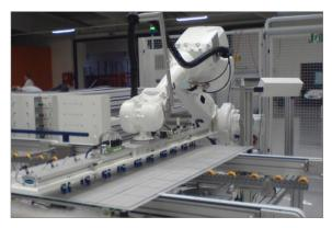
**String Gripper SSG-A** used for the layup of strings on the module/EVA-foil:
