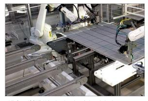
Lift-Cups ISCUP-H for the clamping of glass during layup
