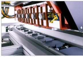
Floating Suction Pads SBS for the handling of wafers
