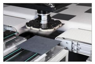
**Wafer Gripper SWG** used for the belt to belt transport of wafers:
