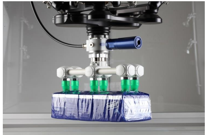
Vacuum End Effector VEE with vacuum generator for handling of bags
