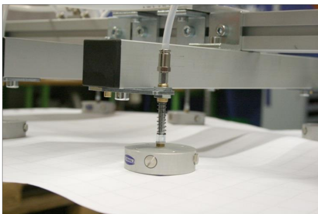
Floating suction cups SBS separated handling of paper
