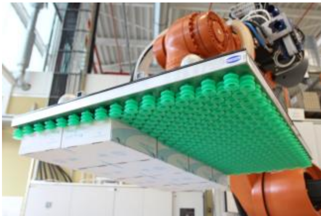
Layer gripping system with e.g. two suction zones for handling cardboard boxes (sheet metal construction with individual dimensions, push-in suction cups)
