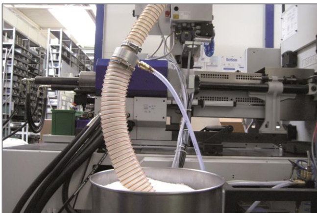
Vacuum generation with feed ejector SEC for transporting granulates
