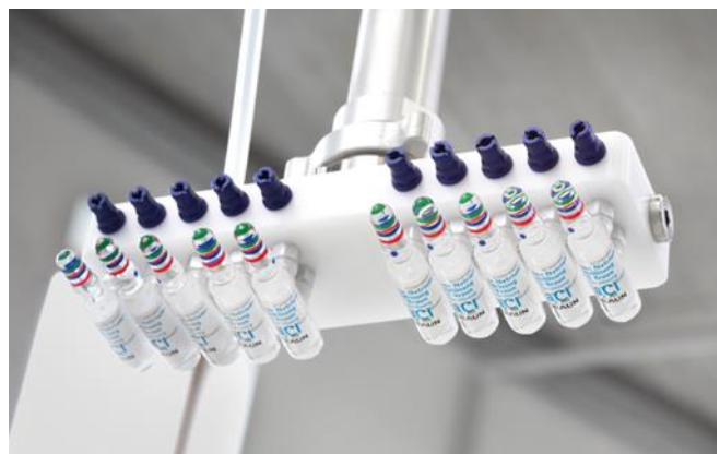
Vacuum end effector for handling of primary packed pharmaceuticals
