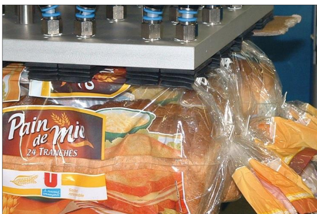
Bellows suction cups FSGB-R for handling of packing materials
