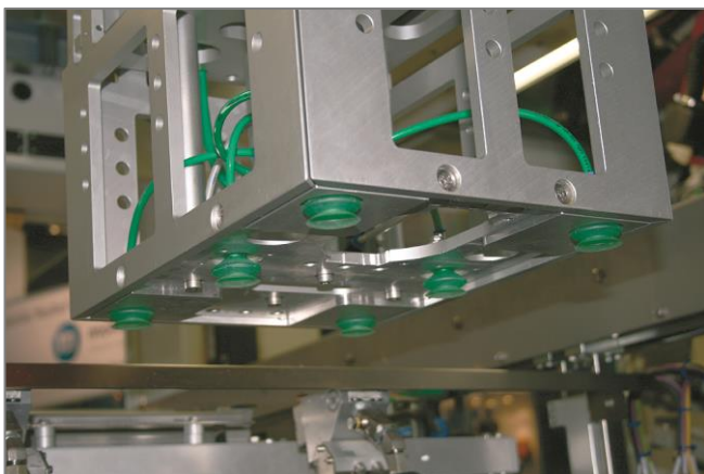
Bellow Suction Cups SPB2 being used in side-loading machines
