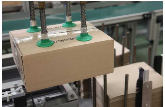
Bellows suction cups SPB1 for handling taped cardboard boxes
