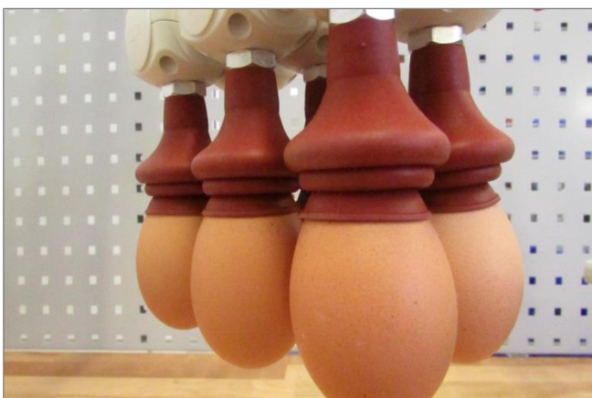
Bellows suction cups FG-X on fresh eggs
