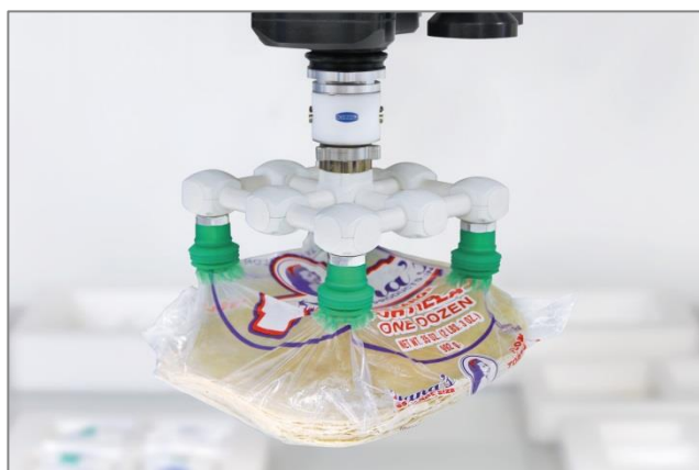
Vacuum end effector with bellows suction cups SPB4f handling pouches with many wrinkles and a low filling degree
