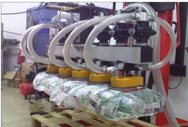
Sack Suction Gripper SG for handling plastic sacks
