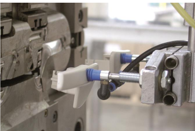
Bellows suction cups FSG being used for hot plastic parts
