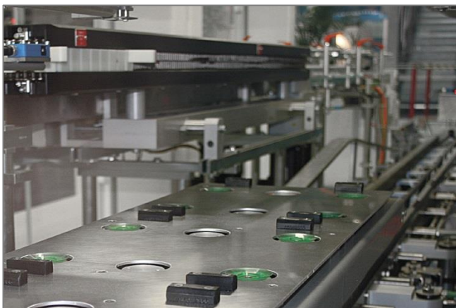
Flat suction cups SPF being used in packaging machines
