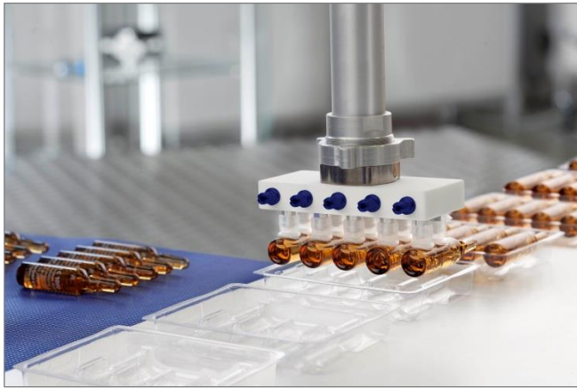
Decentralized vacuum generation by means of ecoPump SEP during the handling of ampoules
