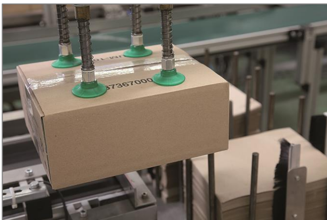
Bellow suction cups SPB1 being used for handling of cardboard
