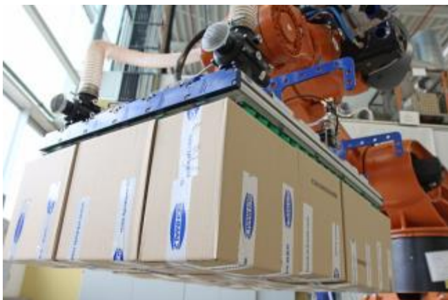
Layer gripping system for handling cardboard boxes and pallets with several suction zones (interlocking construction, push-in suction cups)
