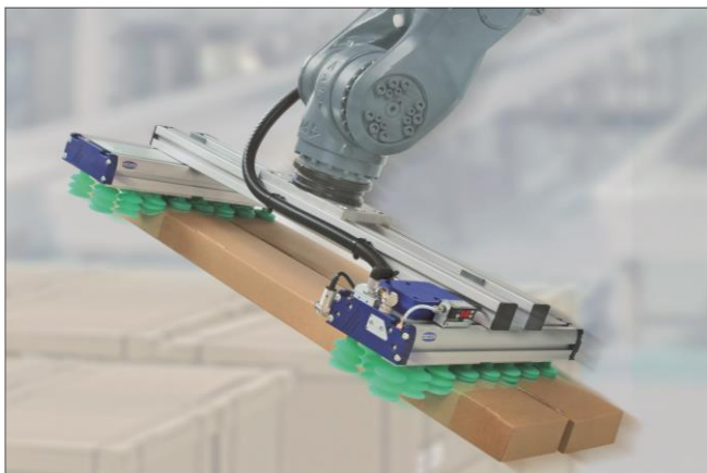
Vacuum area gripping system with two FXP units for handling boxes
