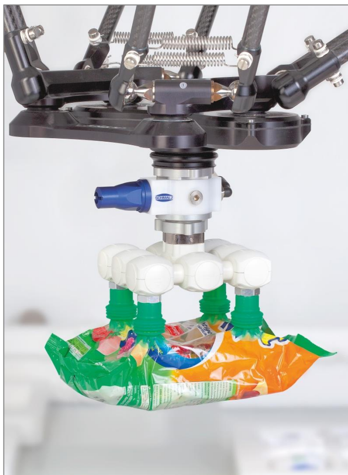
Vacuum end effector with vacuum module and bellows suction cups SPB4f handling flexible bags
