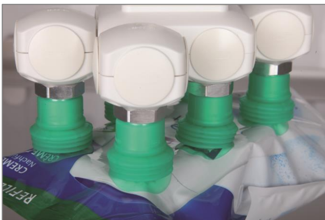
Bellow suction cups SPB4 for handling foil-wrapped products
