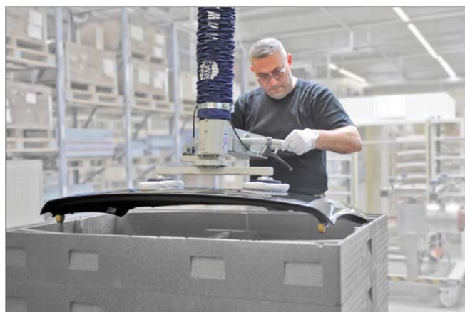
Vacuum tube lifters JumboErgo being used panoramic roof handling
