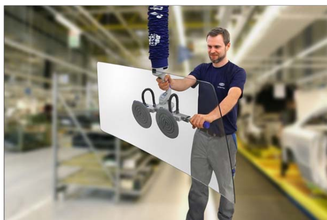
Vacuum tube lifter JumboFlex being used for windshield handling
