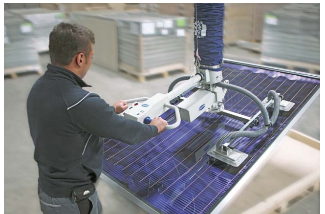
Vacuum tube lifter JumboErgo being used for the module handling
