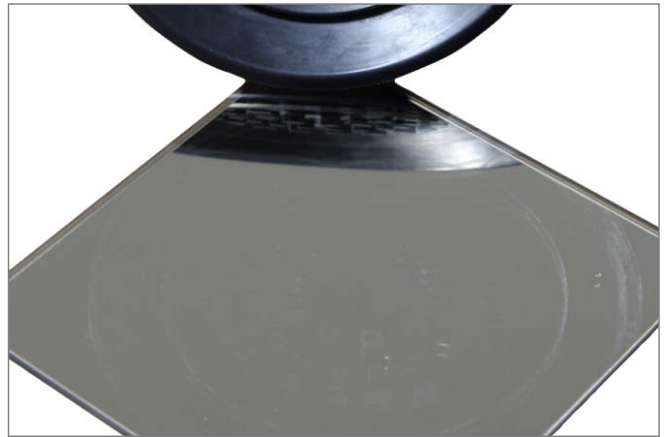
Marking of Nitrile PVC (Commonly used material for glass handling)
