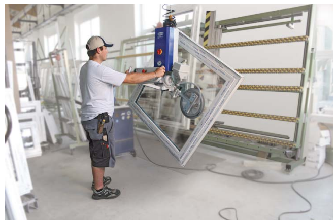
VacuMaster Window being used during the framing of windows
