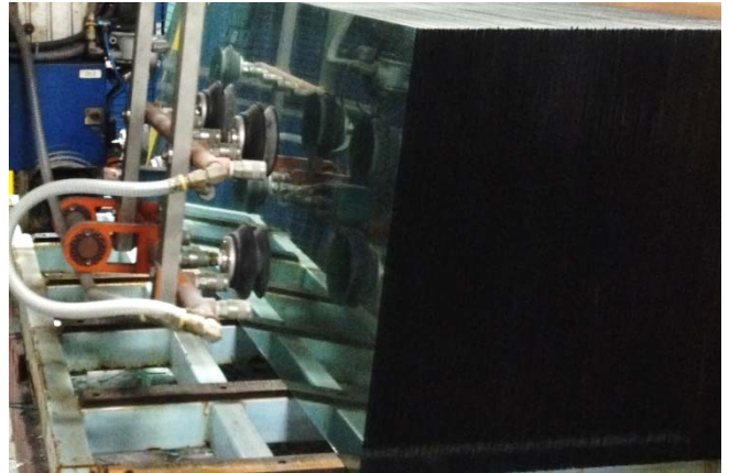
Suction cups FSGA made of Vulkollan being used on destackers
