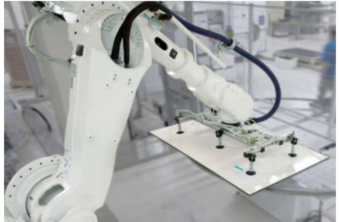
Vacuum suction spider SSP being used for the backsheet layup
