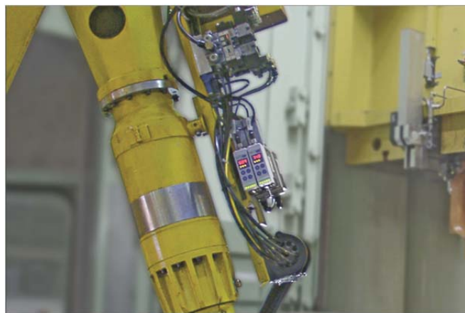
Compact ejector X-Pump used for loading of a bending line
