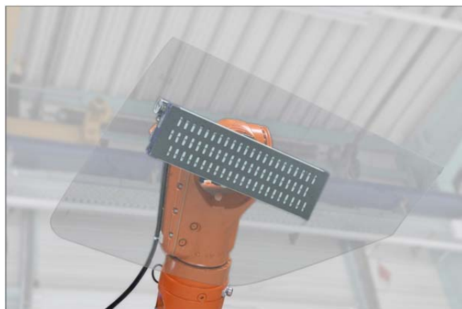
Vacuum area gripping systems FXP used for automotive glass handling
