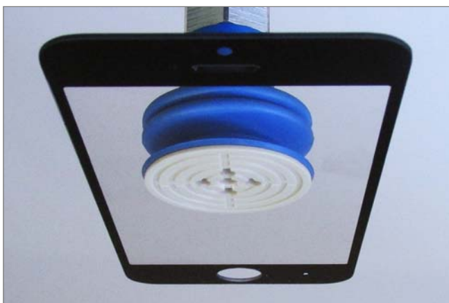
Suction cup inserts SPI PEEK being used for display glass handling
