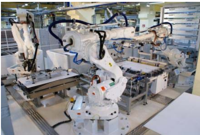
Vacuum suction spiders SSP being used in the framing station
