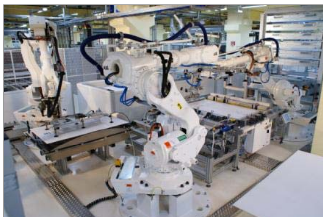
Vacuum suction spider SSP in the framing station of PV modules
