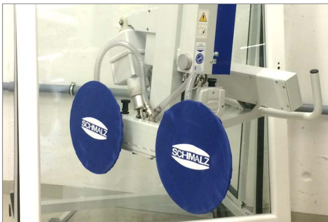
Protection covers PC used on suction plates
