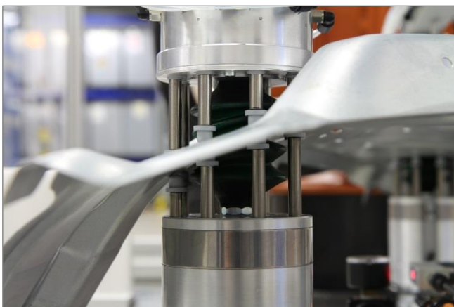
SSCB – handling of a body part
