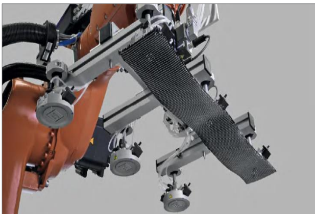
Needle gripper SNG-BV handling composite textiles
