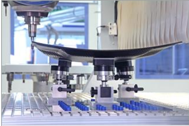
Basic holding fixture BHF for manual 3D clamping
