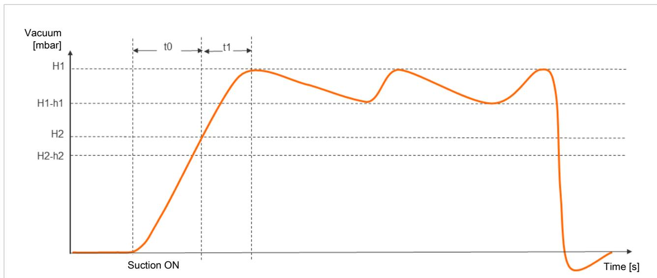
The evacuation time  $t_0$  is defined as the time (in ms) from the start of a suction cycle, which is started by the "Suction ON" command, until switching threshold H2 is reached.
