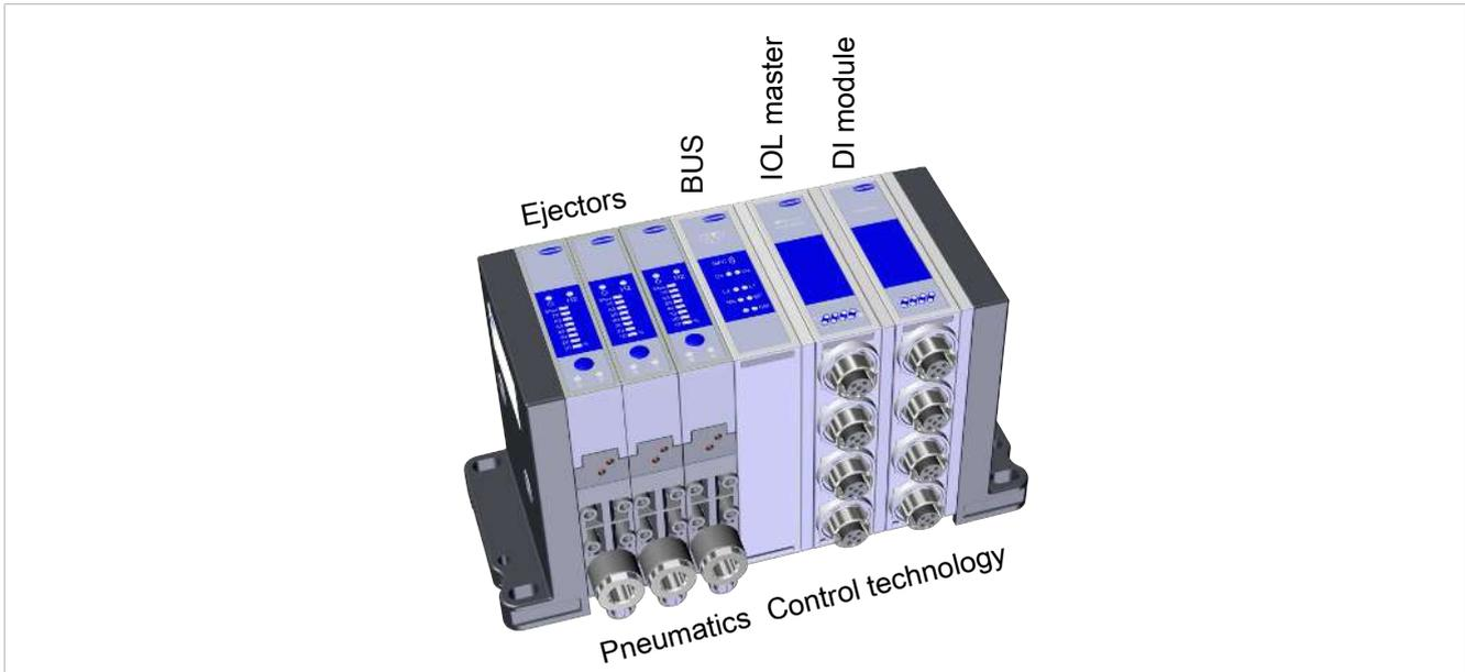
The Schmalz Compact terminal SCTSi, SCTSi for short, is a compact unit consisting of individual discs that links several vacuum generators, ejectors, IO-Link class B masters and digital input modules (DI modules).
