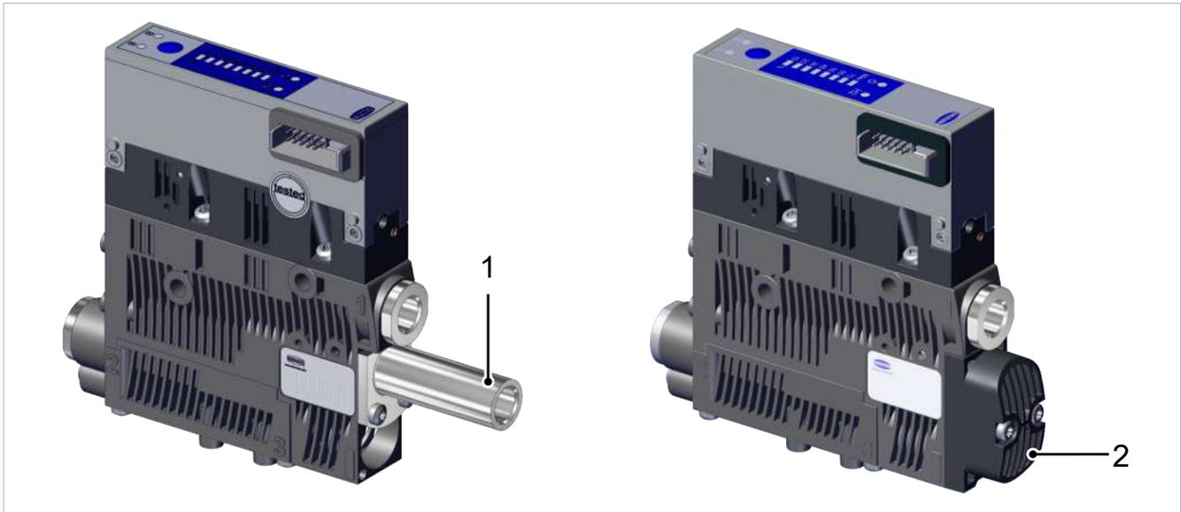
1 Variant with exhaust outlet with **exhaust duct**
