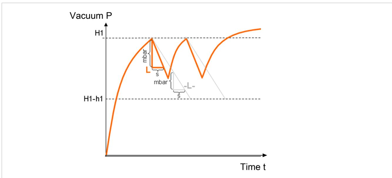
If the leakage is higher than the value, the ejector readjusts immediately. If the permitted leakage is exceeded twice, the ejector switches to continuous suction. The condition monitoring warning is activated and the system status light switches to yellow.
