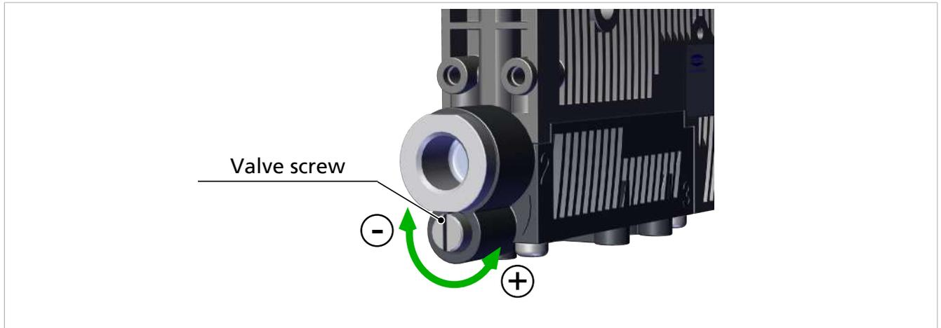
1. Turn the valve screw clockwise to reduce the flow rate.
