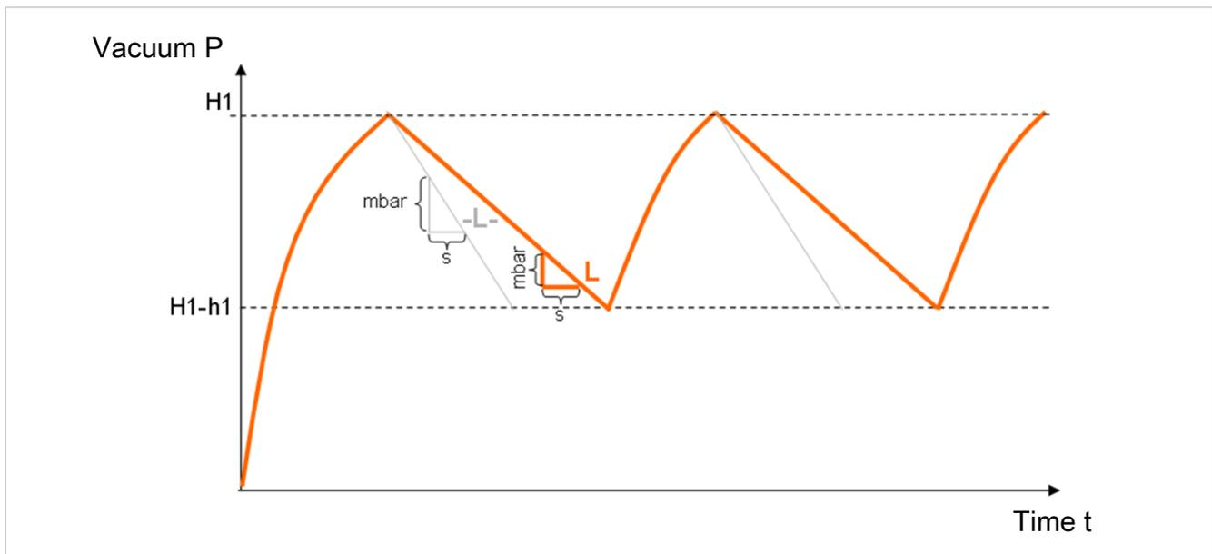
If the leakage is lower than the set value, the vacuum continues to fall until it reaches the switching point  $H1-h1$ . The ejector begins to suck again (normal control mode). The condition monitoring warning is not activated and there is no effect on the system status light.
