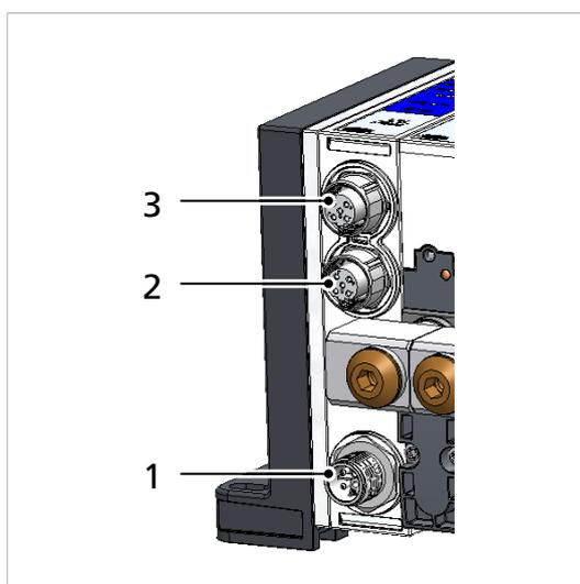
1 M12-L electrical connection plug for voltage supply
