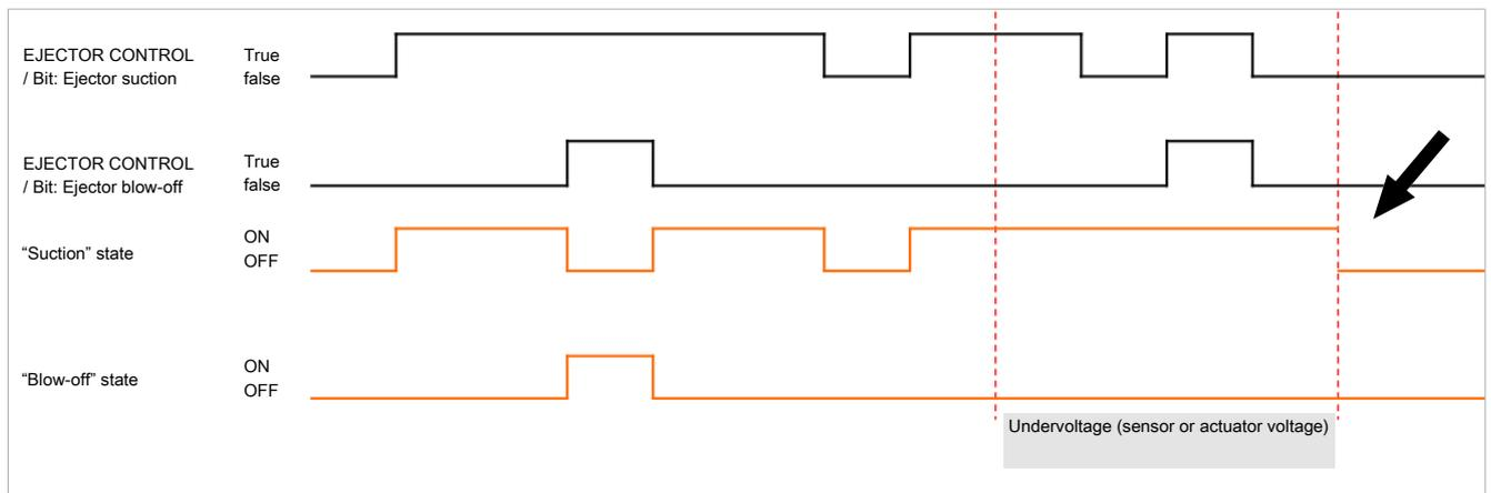
The blow off valve on the ejector is activated and deactivated using the blow off command. The valve is always designed as an NC (normally closed) variant and switches the air pressure channel to the vacuum connection for the duration of activation. If both suction and blow off are activated, blow off is given higher priority and the venturi nozzle is not activated.
