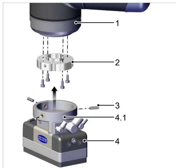
1. Mount the flange plate (2) on the robot (1).
