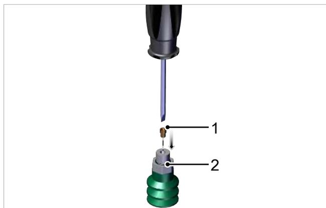
2. Screw the entire screw-in suction cup (1) into the suction plate (2) with a tightening torque of 5 Nm.
