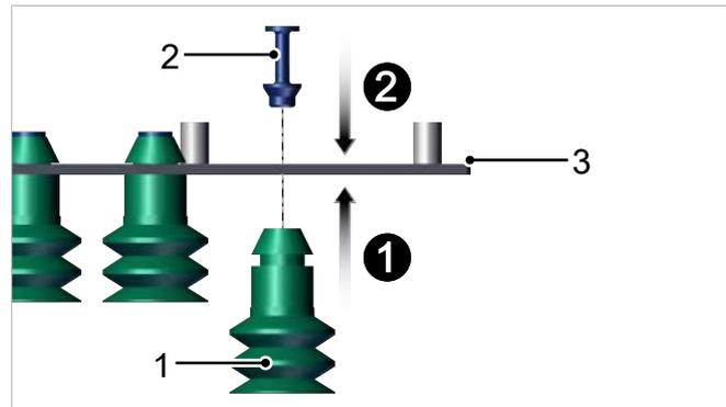
2. Insert the flow restrictor (2) into the plug-in suction cup (1) from above ②.
