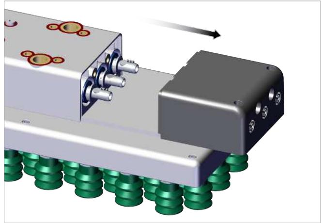
1. Pull out the ejector modules (2 or 3).
