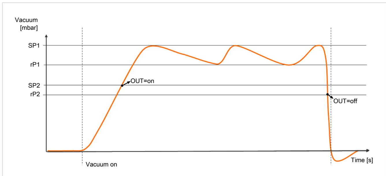
The ejector has an integrated air saving function and automatically regulates the vacuum in suction mode:
