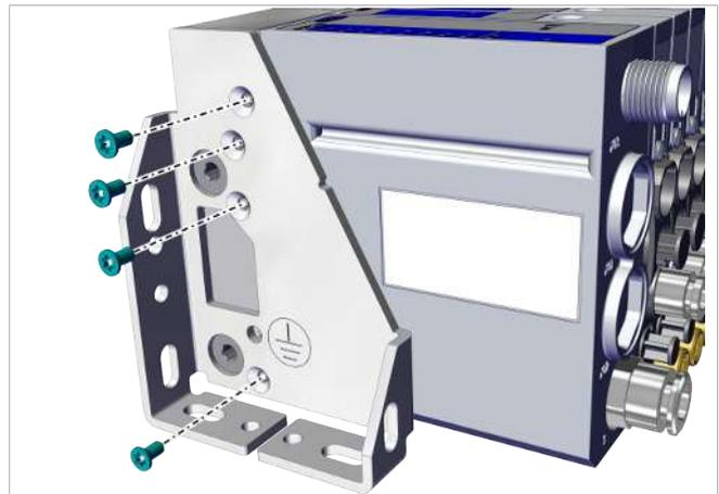
2. Remove the mounting bracket (1) ① and remove the silencer (2) ②.
