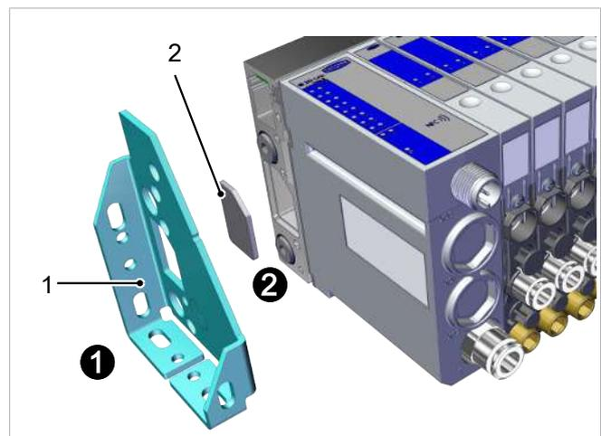
3. Clean the contact surfaces of the mounting bracket and terminal (including the extract air channel if necessary).
