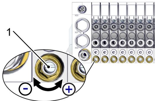
The blow-off flow rate is set to 100% (opened 2 turns) when delivered.
