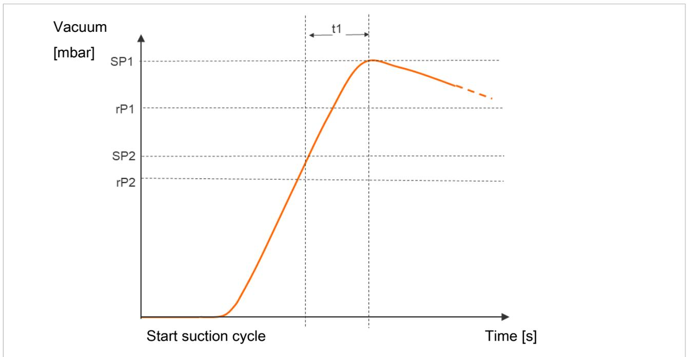
The measured evacuation time  $t_1$  can be read out using the "Evacuation time  $t_1$  for ejectors" parameter 0x0095.
