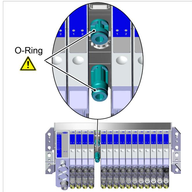
8. Carefully press in the new ejector or valve (2) and printed-circuit board adapter (3) correctly at the free position by hand until they stop flush ①. Check that the three O-rings are positioned correctly and tighten the hex socket head screw (1) with a maximum tightening torque of 2 Nm ②.
