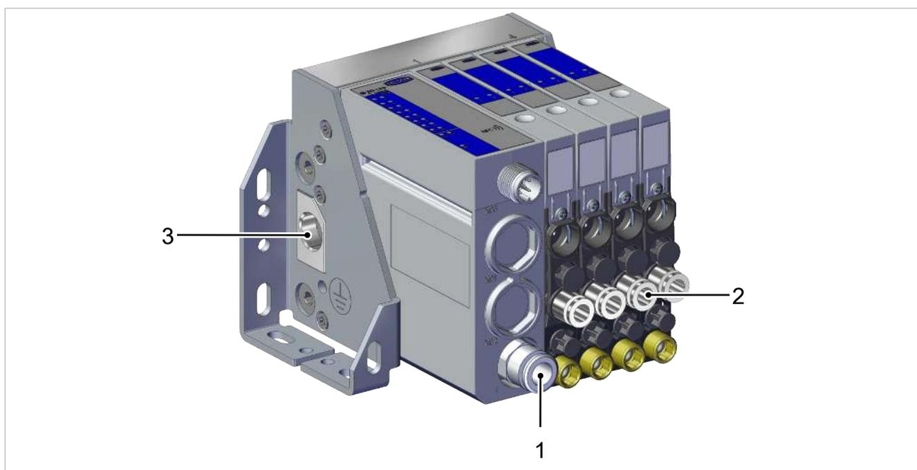
The compressed air connection (1) with plug connector for VSL 8/6 is marked with the number 1.
