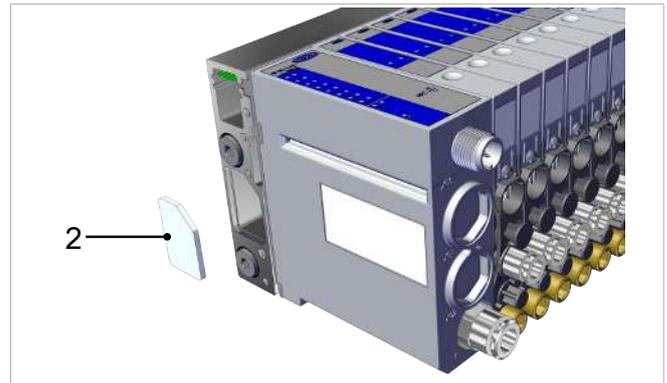
5. Fasten the mounting bracket to the terminal in the correct position using all the screws. Coat the screws with a light-duty thread locking compound and tighten with a torque of 1 Nm.
