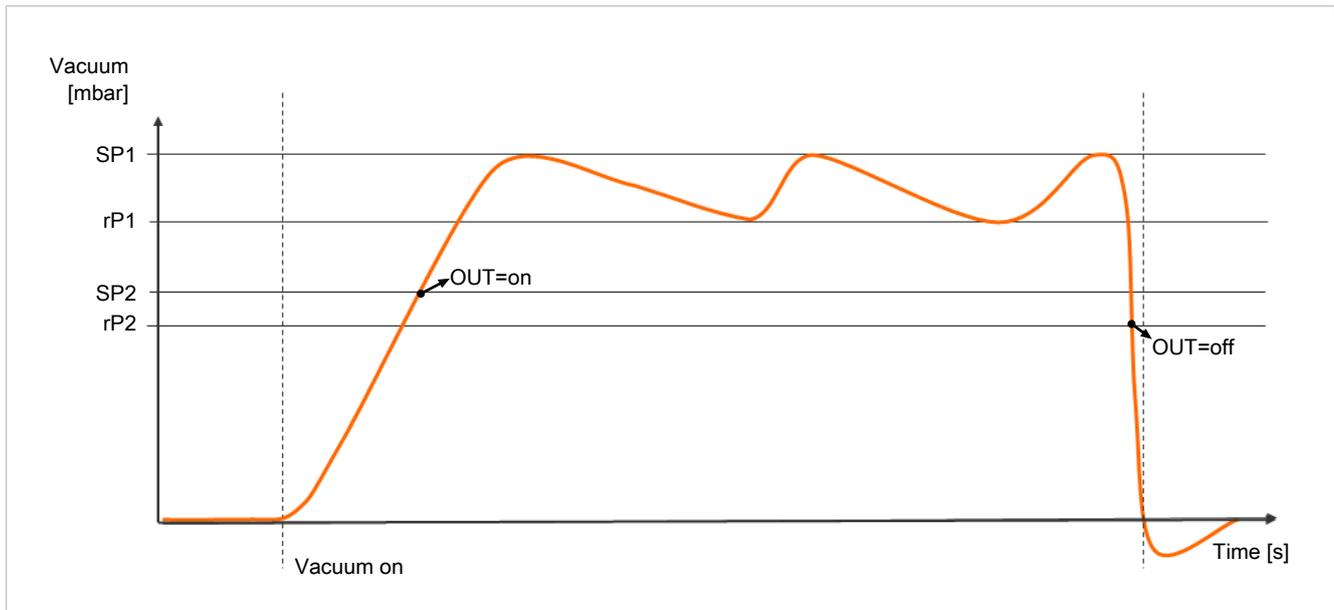
The vacuum valve has an integrated control function and automatically regulates the vacuum in Suction mode:
