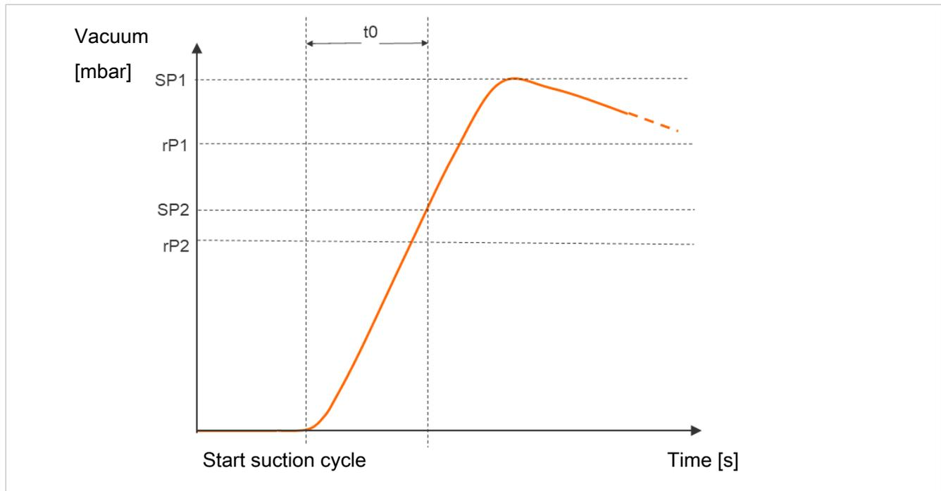
The evacuation time  $t_0$  is defined as the time (in ms) from the start of a suction cycle, which is started by the "Suction ON" command, until switching point SP2 is reached.
