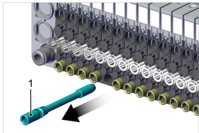
3. Carefully pull the ejector/valve (2) out of the bracket in the direction of the removed screw.
