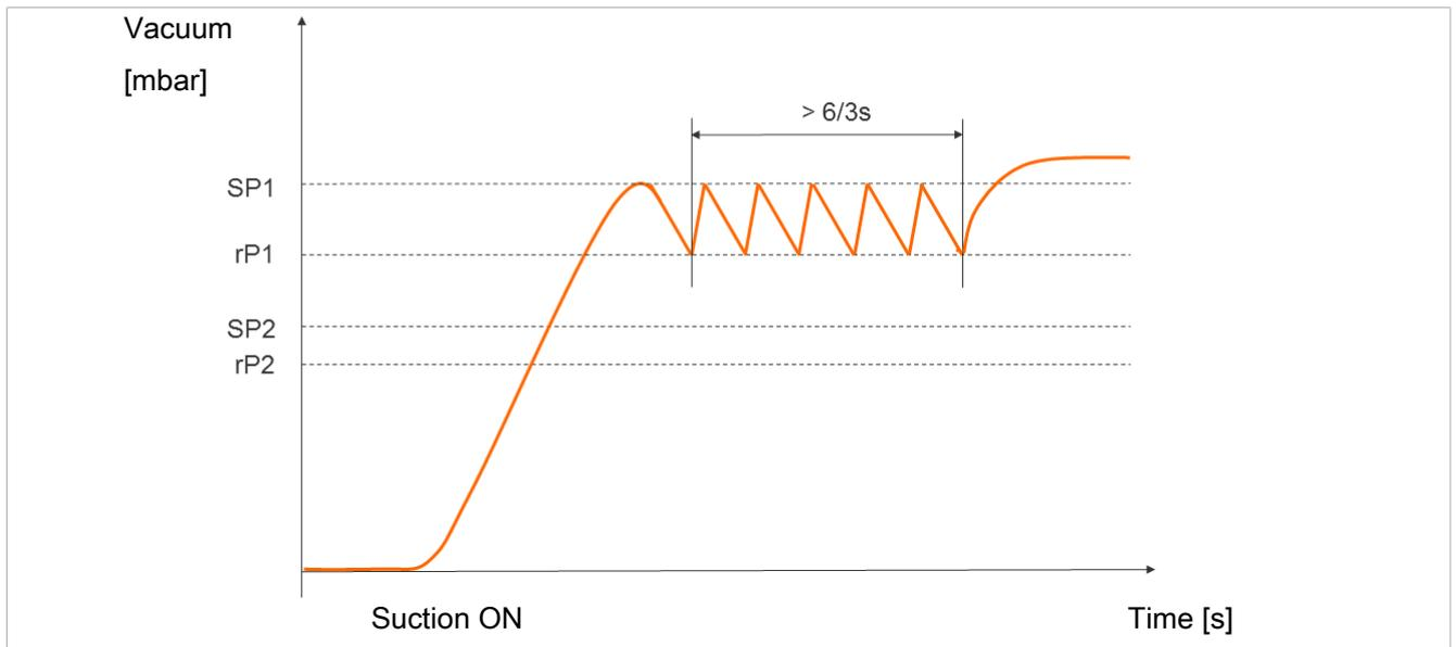
When the air saving function is activated and there is a high leakage level in the gripping system, the component switches between the Suction and Suction off states very frequently. The number of pilot valve switching operations therefore increases rapidly within a short period of time.
