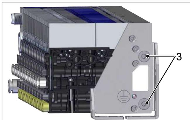
2. Install the mounting element with the 1/8" internal thread (e.g. plug connection) for the compressed air hose.
