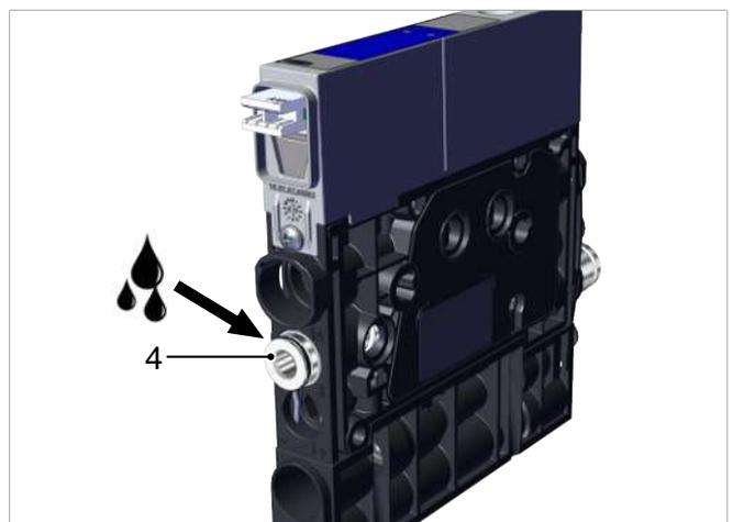
7. Before mounting the ejector/valve or dummy plate, check the position and condition of the O-rings.
